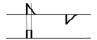
This pulse is then fed to a 555 timer, acting as a <u>Mono-stable Multi-vibrator</u> which gives a 0.8 ms delay. Now this delayed pulse is passed through a NOT gate as we need a rising edge for the shift register. The inverted pulse, when superimposed on the original signal, can easily sample 0's and 1's as shown in following diagram:
